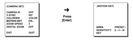
Select ON and press [ENTER] and the MOTION DET additional menu will appear. The AREA menu, selecting the screen area where the MOTION detection function will be applied may be selected by PRESET or USER. Set AREA to PRESET and the MOTION detection function will be applied to the factory default part.
